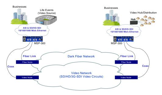
Example Application: IPITEK MSP-300 is used for collecting and aggregating data and video services from local access loops. Data services include 10/100/1000 Mb/s Ethernet and video services include ASI, SD, and HD-SDI. Such services can be carried over Dark Fiber or video circuits at 1.485 Gb/s (HD), 2.97 Gb/s (3G) or 270 Mb/s (SD) for optimized bandwidth and video transport service utilization.
