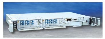
IPITEK is proud to introduce the new IPIswitch Optical Protection Switch. The IPIswitch platform provides a fullymanaged, seamless solution to protecting transmission links against fiber breaks that will cause lengthy traffic disruption. The IPIswitch is compatible with all of IPITEK's digital and analog transport platforms, enabling a low-cost, feature-rich solution for optical path protection. Some key features of the IPIswitch Optical Protection Switch include:
