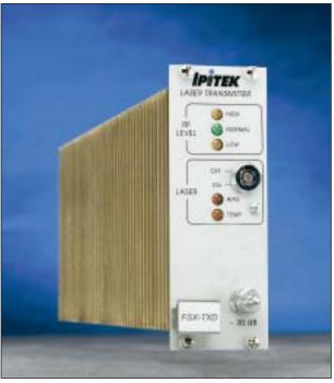
IPITEK's 1310 DFB Laser Transmitter Module is a full-feature direct modulation transmitter for a variety of architectures, including narrowcast and broadband applications. This versatile and compact state-of-the-art transmitter, with its global 860 MHz bandwidth and 80 channel NTSC rating, is one of the highest performance lasers on the market. IPITEK's chassis system houses as many as ten of these laser modules, along with the DC Power Supply and Fan Bay.
