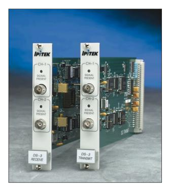
Integrated Photonic Technology (IPITEK<sup>®</sup>) DS-3 converter modules are used in conjunction with IPITEK IMTRAN<sup>®</sup> CQ Series transmission systems to transport T3/E3 data communications over fiber. This product takes advantage of the increasingly popular T3/E3 format with applications ranging from T3/E3 broadcast video and MPEG compressed video to small telephone systems.
