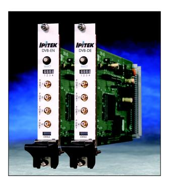
The IPITEK HBR-DVB provides Quad DVB-ASI ports per module. It allows transmit and receive up to 4 independent DVB-ASI per module or 600 MPEG-2 or 122 HDTV per wavelengths via the HBR-2502 digital transport system.
